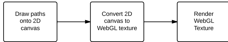
Figure 5.7: Process of drawing lines and annotations onto a WebGL canvas using a 2D canvas
