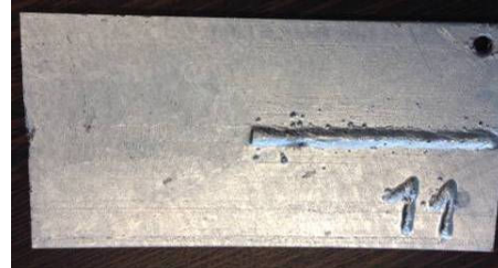
Figure 3: Galvanized grinded and non-grinded weld with ZINQWeld
