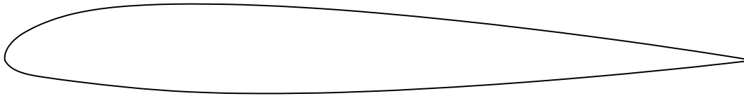
Figuur C.1: NACA23012, dikte: 12%
