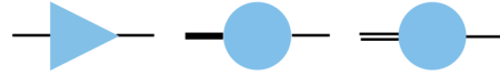
Figure 2.2: Possible ways to depict differences in the bond dimension. The bond dimension is higher on the left side than on the right side.
