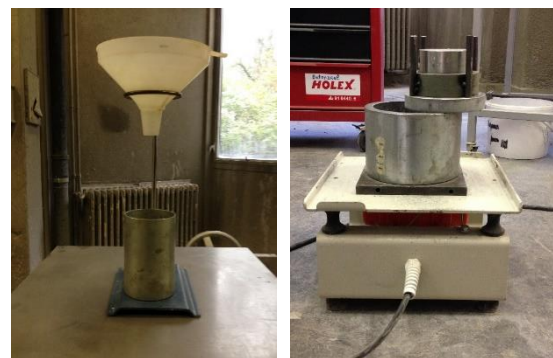
Figure 1: Test setup gravity test (on the left) and compaction test (on the right)
