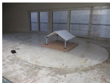
Model placed in the middle of the turn table and secured by angle profiles and screws; pitch roof
