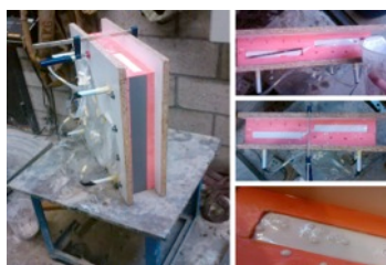
Pour up the mould with IPC matrix on the vibration plate to remove internal air bubbles and improve the pouring process
