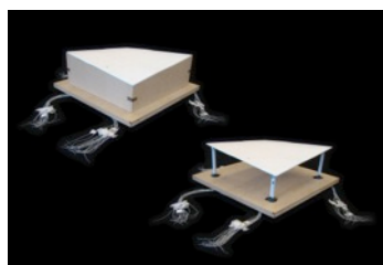
Remove mould after post curing; cut protruding PVC air tubes; polish model surfaces; poste model onto wooden base and make walls
