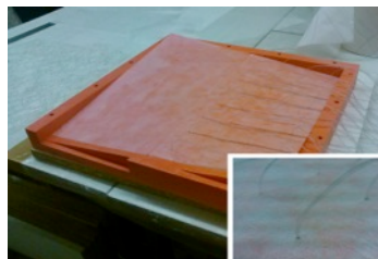
Place and impregnate 30 gr/m 2 glass-fibre mat
