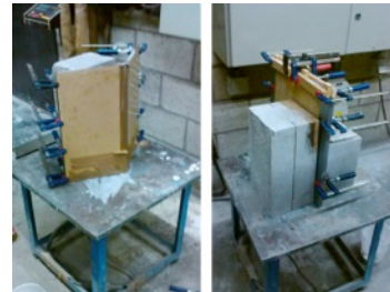
Pour up mould with IPC matrix on the vibration plate to remove internal air bubbles and improve the pouring process; left: pitch roof; right: flat roof
