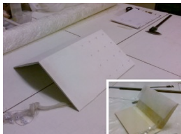
Remove mould after post curing; cut protruding PVC air tubes; polish model surfaces; additional glass-fibre membrane of 30 gr/m 2 to smoothen surfaces of pitch roof
