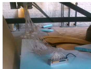
Scanivalve placed underneath the wind tunnel; connection of the redirected PVC air tubes to the Scanivalve pressure sensors
