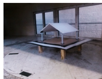
Duo-pitch canopy elevated on four columns of 150 mm; addition of an aerodynamic wing (free flow field test case)
