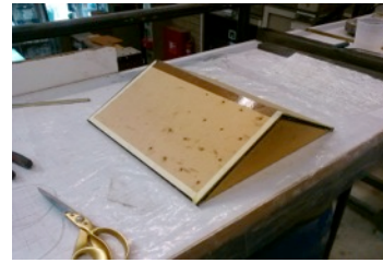
Assemble mould from the laser cut faces and grease mould; pitch roof
