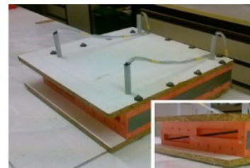
Close the mould and secure from leakage by bolting both mould parts together; the wooden sheets prevent damaging the mould itself
