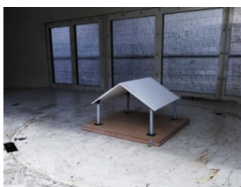
Duo-pitch canopy placed directly onto the turntable of the wind tunnel (boundary layer test case; section 4.2.4.1 and 4.2.4.2)
