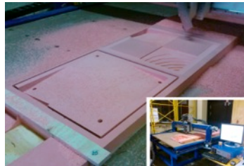
CNC mill the mould layers; bottom layer after finishing operation; top layer at roughing operation
