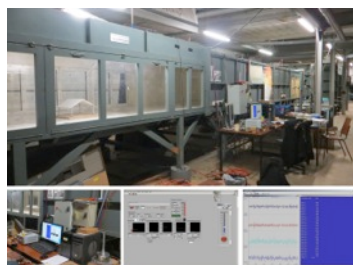
Wind tunnel experiment set-up, computer control, LabView software; pitot measurements; Motor drive; Scanivalve measurements
