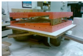
Redirect PVC air tubes at the top side through the columns in a pattern that avoids cleching the tubes by closing the mould
