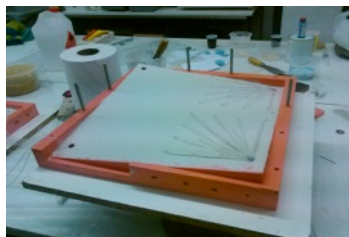
Redirect PVC air tubes at the bottom side through the columns in a pattern that avoids cleching the tubes by closing the mould
