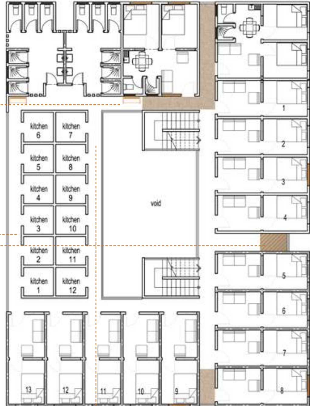
Floor plan of the second floor as designed by Asare (the final implementation is slightly different) First floor is similar but with less improvements made by the residents.
