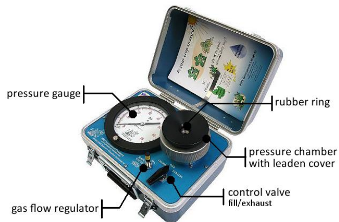
Figure 2.6 Portable Scholander pressure bomb
