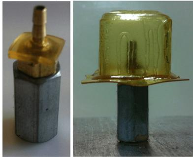
Figure 6.8: A tiny hole was made in the bottom plane of the 3D cubic part, through which a small metal tube, with a diameter of 2 mm, inserted. The metal tube is screwed on a connector part.
