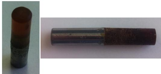
**Figure 5.9:** Self-Healing part after the temperature/press process described in steps: 1 to 4. a) Top View and b) Side View.
