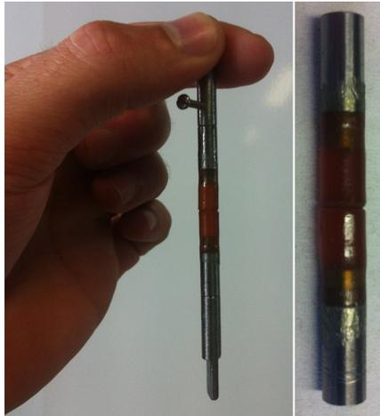
**Figure 5.16:** Pictures of the SH-parts which are joined together after the self-healing process in the mechanical fuse.
