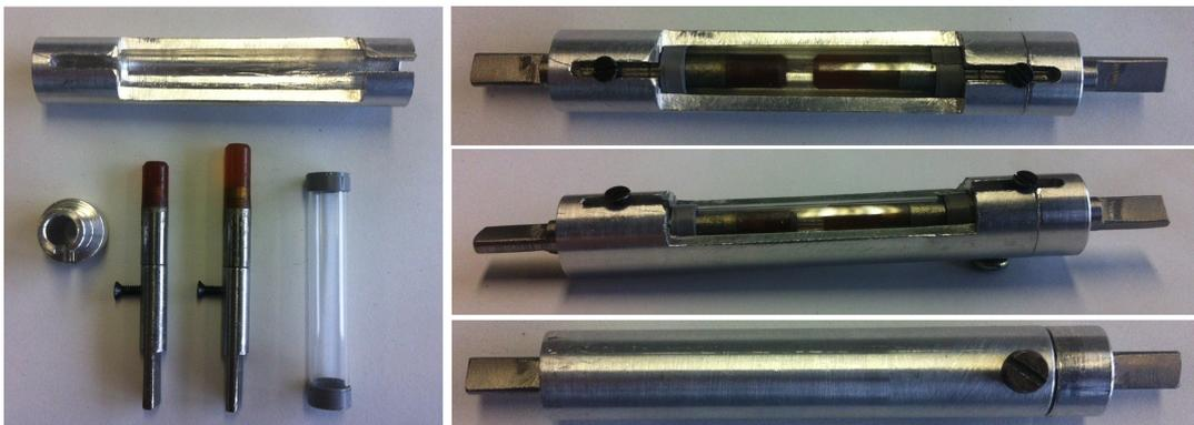
**Figure 5.6:** Left: Picture of the parts of the Self-Healing mechanical fuse. Right: The assembled Self-Healing Mechanical Fuse: top view, side view and bottom view.
