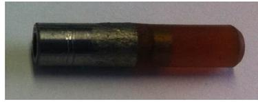
Figure 5.10: SH-part with chamfer on the edge.
