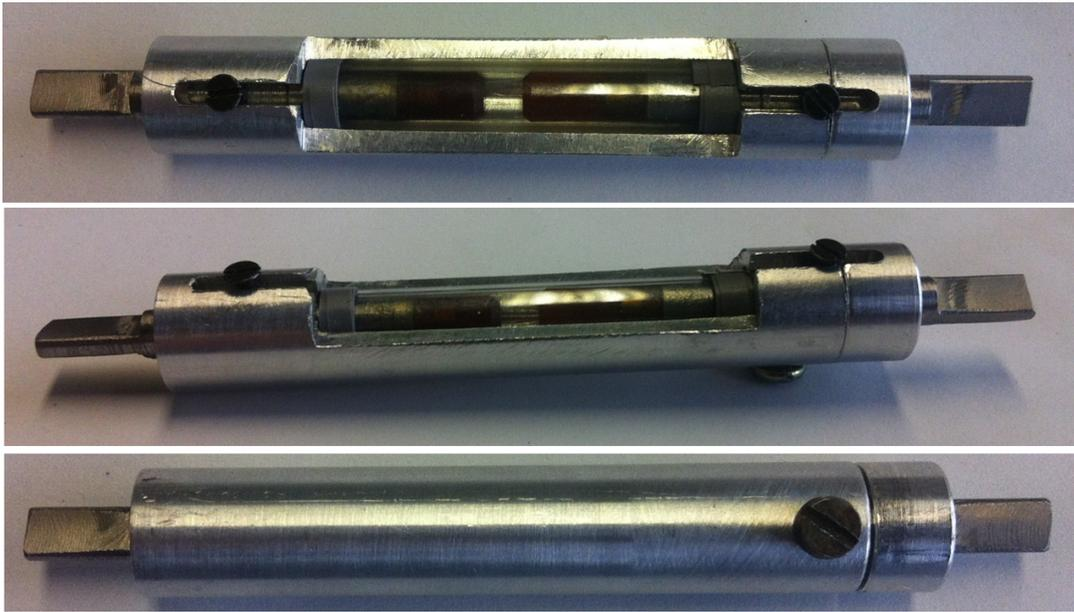
**Figure 23:** Self-Healing Mechanical Fuse (SH-MF). This fuse is not subjected to a first self-healing cycle yet. a) Upper View, b) Side View and c) Bottom View
