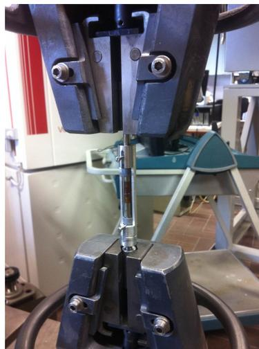
**Figure 5.18:** The SH-MF which is placed between the clamps of the Universal Testing Machine (UTM).
