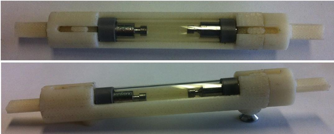
**Figure 21:** 3D printed Prototype of the Self-Healing Mechanical Fuse (SH-MF)
