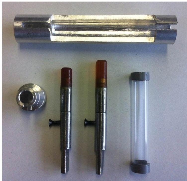
**Figure 22:** Parts of the Self-Healing Mechanical Fuse: two SH-Assemblies, formed with the components of figure 23, Glass Tube, Aluminum Cover (two parts).
