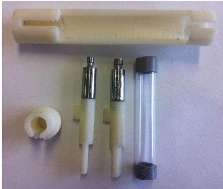
**Figure 20:** The components of a 3D printed Prototype of the Self-Healing Mechanical Fuse (SH-MF): 2 pins with a T-end, a glass tube, ABS-cover (two parts).
