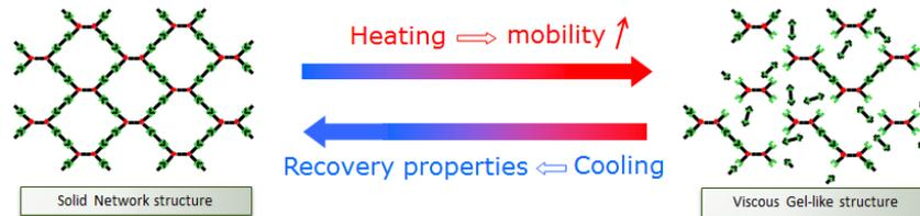
**Figure 4.7:** Equilibrium Diels-Alder reaction, function of temperature. At low temperatures the network is formed due to a high conversion to Diels-Alder bonds. At elevated temperatures a lot of Diels-Alder bonds will break, the conversion will drop and the mobility of the polymer chains will increase. At relative high temperature the polymer will receive a gel-like structure.
