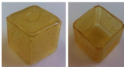
**Figure 6.4:** Cubic part after being naturally cooled down in the oven and removed out of the cubic mold: Side-Top View and Side-Bottom View.
