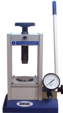
**Figure 14:** Picture of the manual hydraulic press used for the shaping proces of the DPBM-FGE-J400 SH-part, which is used in the SH-Mechanical Fuse: Specac: Atlas 15T Manual Hydraulic Press [9].
