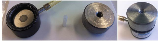
**Figure 5.8:** Left: Different parts used for pressing the porous polymer powder into a cylindrical Teflon tube, from left to right: Bottom part, Teflon tube and steel holder. Right: The parts assembled. The powder can be poured into the Teflon tube and using a steel press pin this powder will be pressed into a cylindrical part in the hydraulic press.
