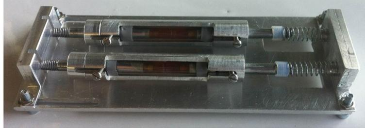
**Figure 5.15:** Holder with soft springs, in which the SH-MFs can be inserted. Due to the soft springs the SH-parts are gently pressed together in order to gain maximal contact between the two contact surfaces during the SH-process.
