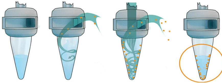
**Figure 1.9:** Scheme clarifying the Coriolis®  $\mu$  air sampling principle. A sterile cone containing the collection fluid is screwed into the sampler device. During sampling, air is sucked into the collection cone and suspended particles are pulled into the collection fluid, through the centrifugal force of the swirling air. After collection, the particles are contained inside the cone. Reference: Bertin technologies (2008)
