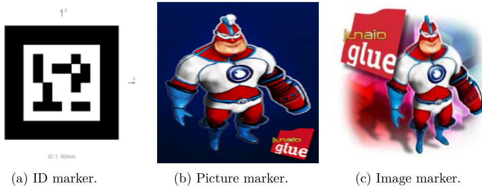
Figure 5.4: Three sort of markers that can be used in the tracking configuration of the Metaio SDK.
