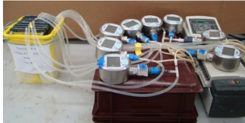
Figure 21 Set-up of the CWP measurement of the membrane modules.
