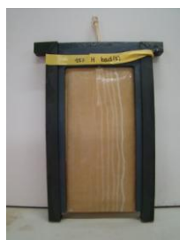
Figure 22 Membrane sampling. Each vertical line corresponds to a sampling moment. The same pattern is present at the back side of the module.
