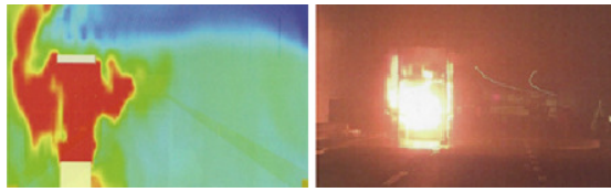
Figure 4 – Comparison of CFD temperature field and Craeybeckxtunnel video measurements.
