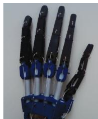
Figure 102: Final product of the anthropomorphic 20-DOF robotic hand [48]
