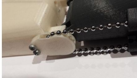
Figure 129: Fixed attachment on the palm for wrist extension and flexion
