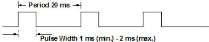
Figure 215: PWM control of an analog servo motor [servocity.com]
