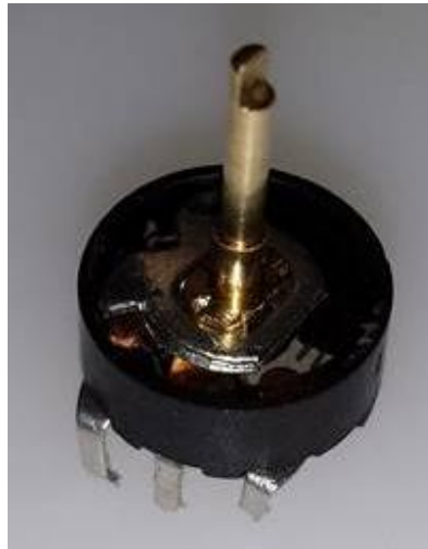
Figure 219: Mechanical constraint on the servo potentiometer axis
