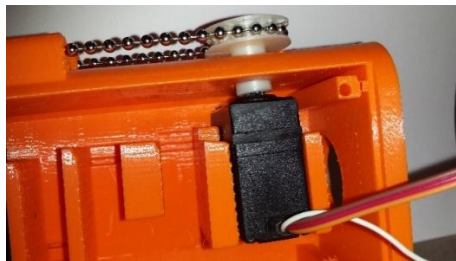
Figure 130: Gear on the motor for wrist extension and flexion
