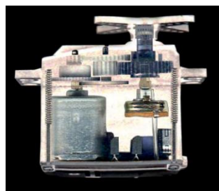
Figure 35: A RC servo motor [Princeton.edu]
