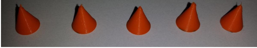
Figure 85: Visual comparison of every setting. From left to right: Fast print, normal print, high quality, ultra-quality and our custom settings
