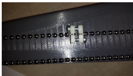
Figure 131: Tension mechanism used for the ball chain
