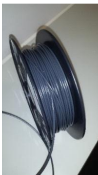
Figure 94: Badly wrapped spool of filament
