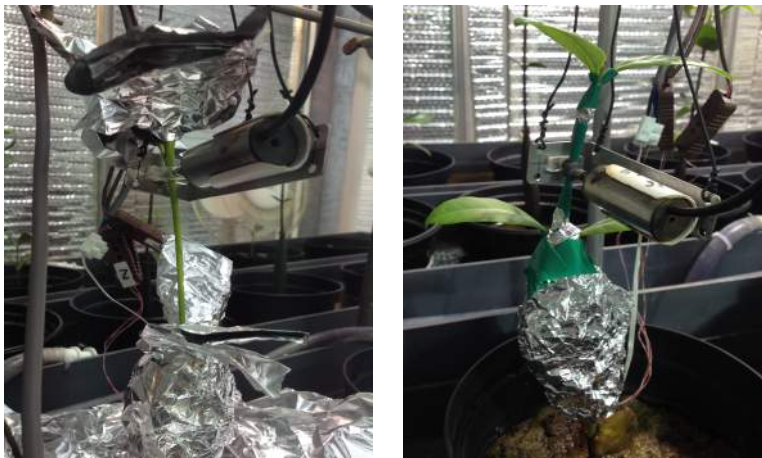
Figure 2.7: Left: Assessing stem water uptake (SWU) by an artificial rain event on plants with covered leaves and soil. Right: Plants with covered stems in order to assess foliar water uptake (FWU) without SWU. Roots were only covered during artificial rain events in order to avoid additional anoxic conditions. Part where linear variable displacement transducer (LVDT) sensor touched the plant was not covered during the experiment.
