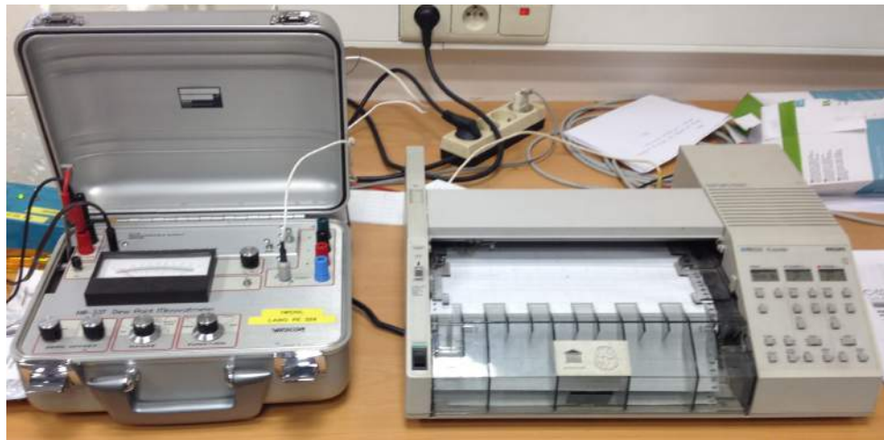
Figure 2.9: The thermocouple-psychrometer (HR-33T, ELITechGroup Wescor, Logan, United States of America) on the left and the strip chart recorder (PM8262, Philips, Eindhoven, Netherlands) on the right.
