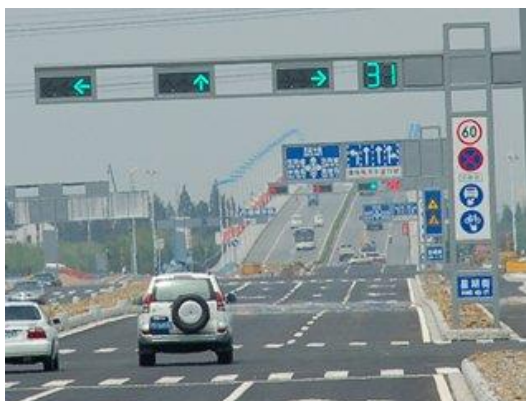
Figure 6 Countdown timers for the green and red phase.
