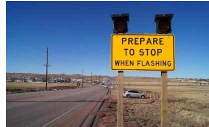
Figure 5 An advanced warning flasher.
