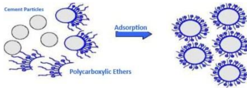
Figure 7-5: Steric hindrance by PCE superplasticizers
