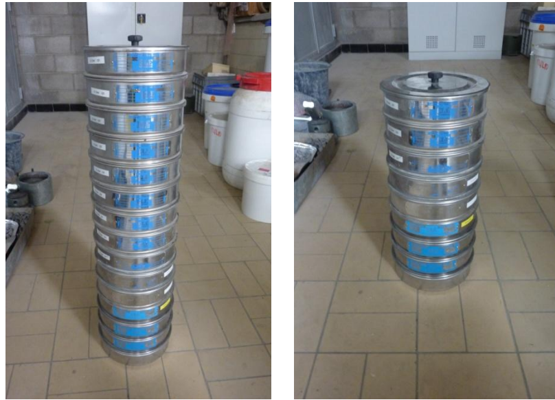
Figure 5-1: Pile of sieves for limestone aggregates (left) and sands (right)
