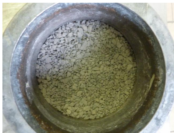
Figure 5-5: A compacted limestone aggregate
