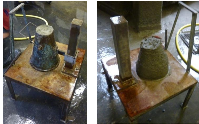
Figure 6-1: Slump test before and after lifting the cone of Abrams
