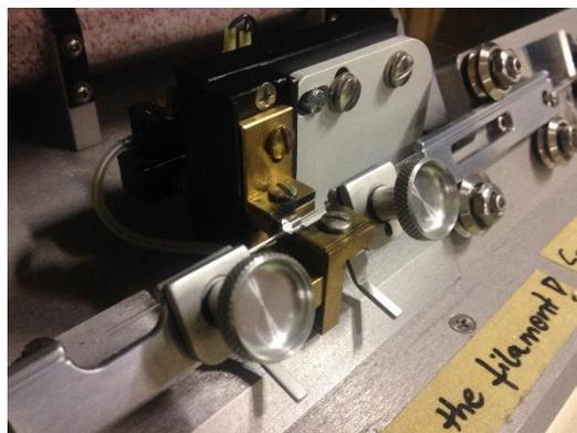
**Figure 9: Needle puller.** Close-up of the p-87 needle puller.
