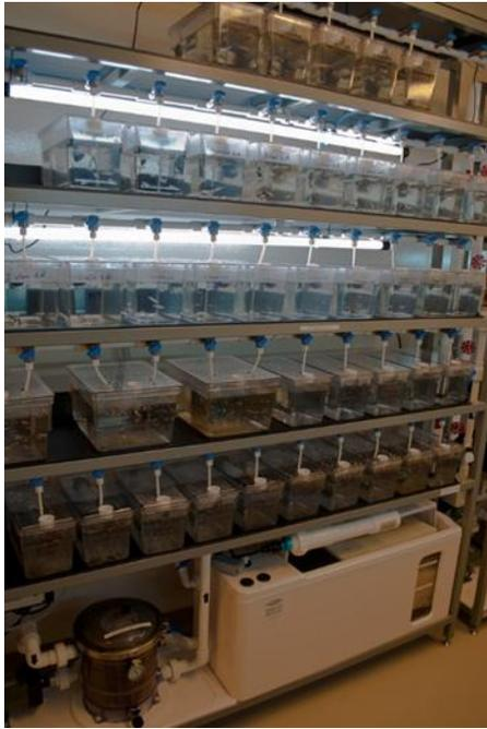
**Figure 8: Marine biotech recirculating system.** Water is moved from the housing tank through a series of components that reduce or remove the waste products. These components include mechanical, biological and chemical filtering units.
