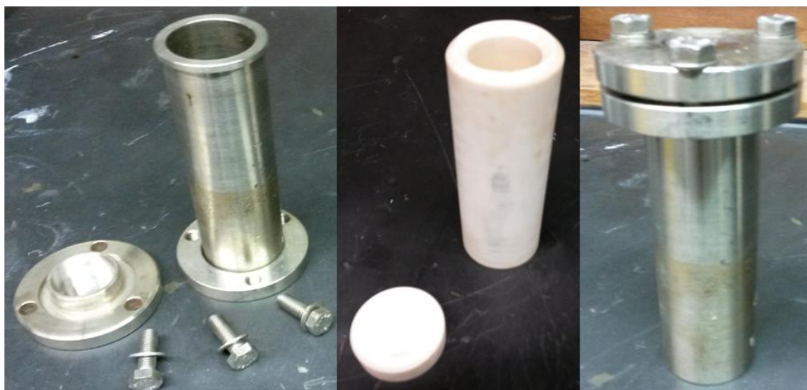
Figure 14: Steel autoclave, Teflon reaction tube and sealed setup.
