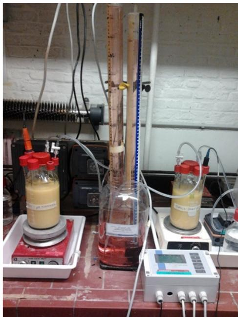
**Figure 4.** Experimental set-up of the semi-continuous batch reactor. Gas tubes with acidic solution can be seen in the middle. Prominent pH controller visible in the back, Consort pH controller in front.
