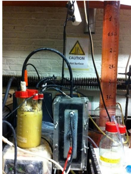
**Figure 5.** Set-up of fermenter with electrochemical extraction cell, pH controller with bottles and gas trap
