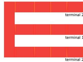
Fig. 8. Layout of a 50 pH shorted stub inductor
