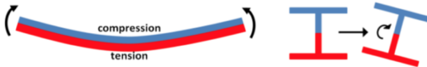
Figure 2.9: Lateral-torsional buckling of beam loaded in strong-axis bending. Extracted from (Sonck et al., 2012).
