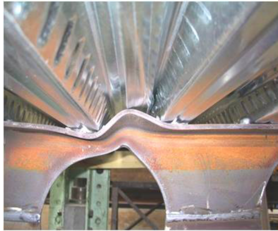
Figure 1.5: Vierendeel mechanism with formation of plastic hinge. Extracted from (Durif et al., 2013).
