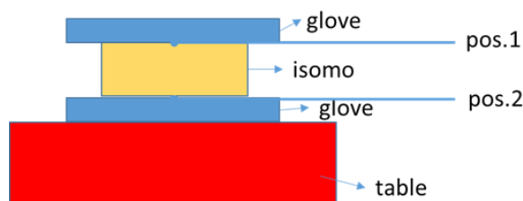
Figure 55: Scheme for experimental set-up for glove with insert
