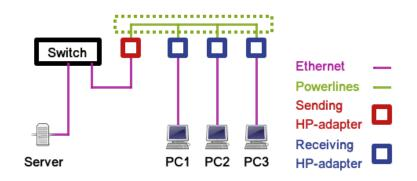
Figure 4.7: Multicast streaming – setup
