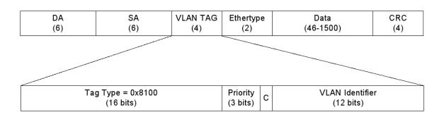
Figure 2.4: VLAN tag structure
