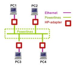
Figure 4.8: Four-node test – setup
