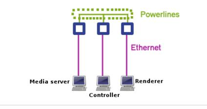
Figure 5.1: UPnP with Topcom adapters – setup
