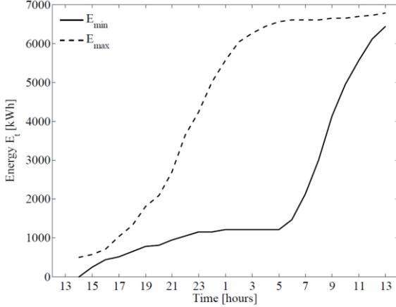
Figure 2: Flexibility profile for charging a fleet of 1000 electric vehicles. The first EVs arrive at 2 pm and the last leave at noon of the following day. Total demand is 7MWh.  $E_{\min}$  and  $E_{\max}$  define the flexibility profile of the aggregator.
