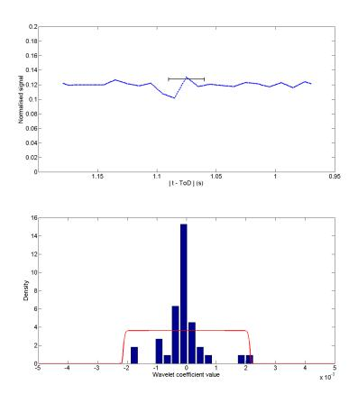
Figure 2.5: Processed time derivative of the poloidal beta, accompanied by the statistics of the wavelet coefficients for a time window of 30 ms.
