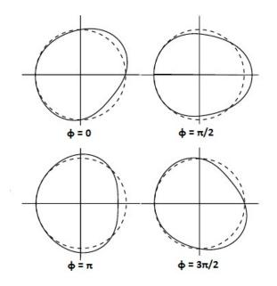
Figure 1.5: A contour plot of the shape of the ballooning-kink mode in the high- $\beta$  limit for four poloidal cross-sections. The kink shape is clearly situated at the outward radial part of the plasma [10].
