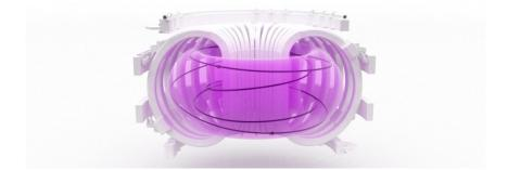
Figure 1.4: A magnetic field line circling around the plasma in a tokamak [28].
