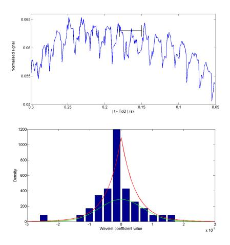
Figure 2.4: Processed plasma current, accompanied by the statistics of the wavelet coefficients for a time window of 30 ms.
