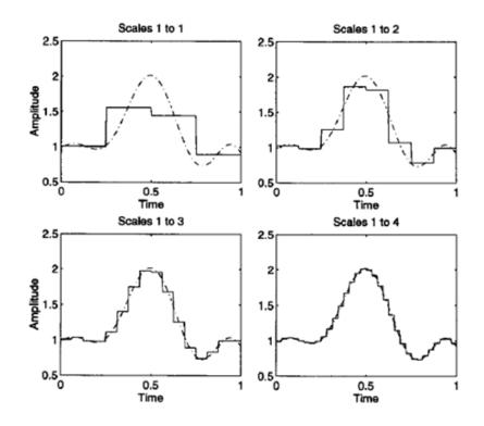
Figure 2.3: Wavelet decomposition of a time signal at four different decomposition levels. The original signal is shown by the broken line. The wavelet reconstruction is given by the solid line [36].
