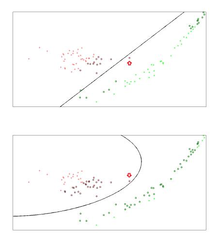
Figure 2.9: Example of the separating hyperplane in two cases. Top: non-separable linear SVM. Bottom: separable non-linear SVM (RBF kernel,  $\sigma = 2$ ). Support vectors are shown by black circles.
