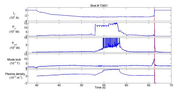
Figure 1.6: Temporal evolution of five predictor signals. The disruption time is indicated by a full red vertical line.
