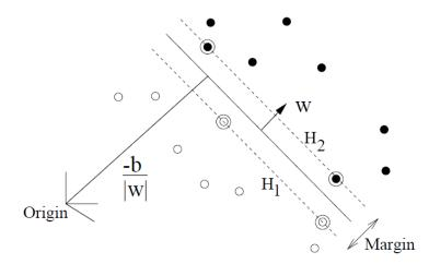
Figure 2.8: A two-dimensional example of a hyperplane separating the two classes in the linear separable case [43].
