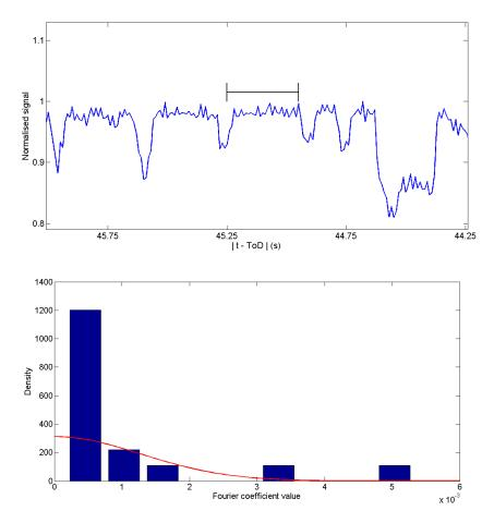
Figure 2.1: Processed total input power, accompanied by the statistics of the Fourier coefficients for a time window of 30 ms.
